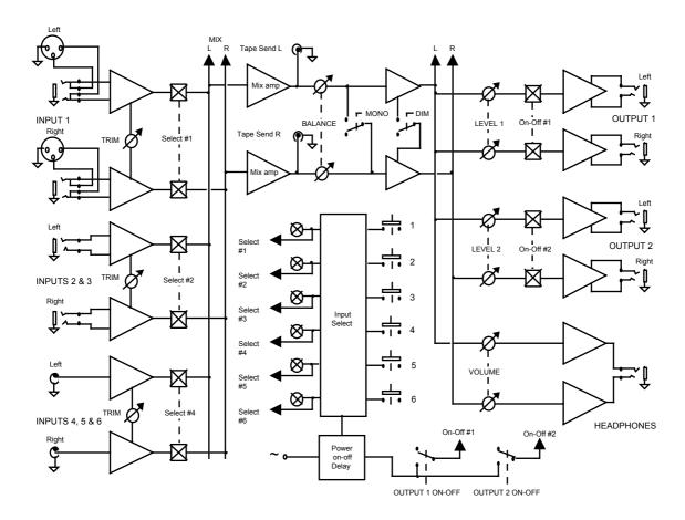
Fig 6.1.1 SPX20 block diagram showing main signal paths
